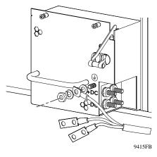
8. Disconnect the grounding cable from the ground lug on the power supply.
